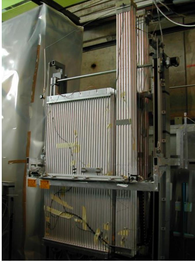
Figure 4.7: The mechanical setup in the GIF area. The BIS is on the left, the two bundles on the right. In the middle it’s possible to distinguish the movable support of the two ^{241}\text{Am} sources.
